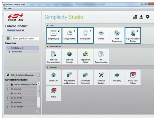
2. A configurator tool provides users with a graphical interface and properties windows. Customers can designate port pins as capacitive-sensing inputs and configure library performance settings.
