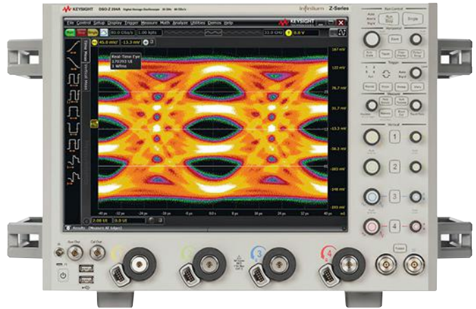
PAM-4 has four distinct levels to keep cables at four 50 Gbaud connections to deliver 400 Gbit/s Ethernet (as shown on Keysight's real-time oscilloscope running N8827B PAM-4 analysis software).
